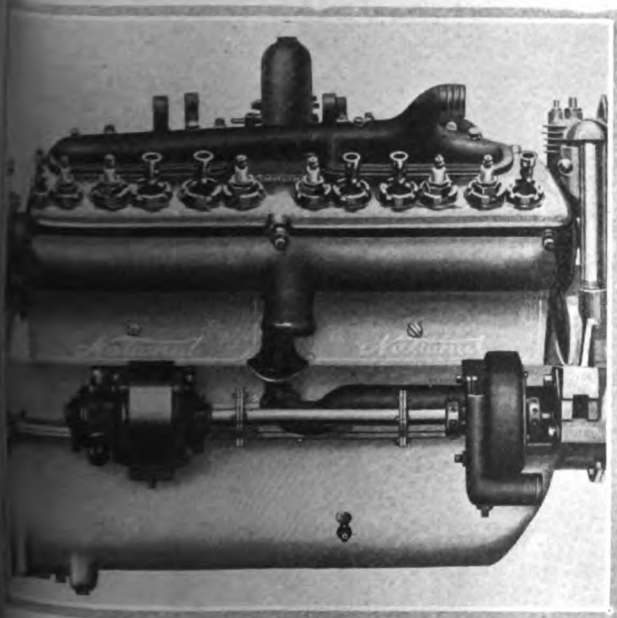
Right side of National twelve, showing mounting of pump and generator, the only motor accessories not located in the V
